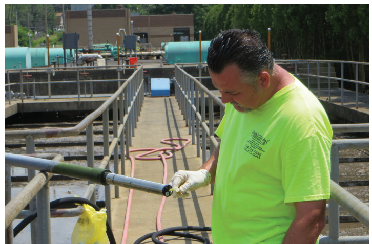
Vince Cappitte cleaning a VARIION ISE probe
